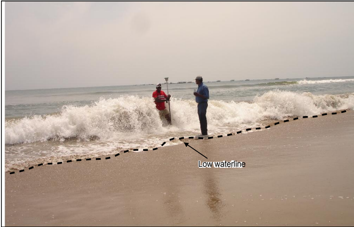
Fig. 7.34a: DGPS survey at Low Tide Level
