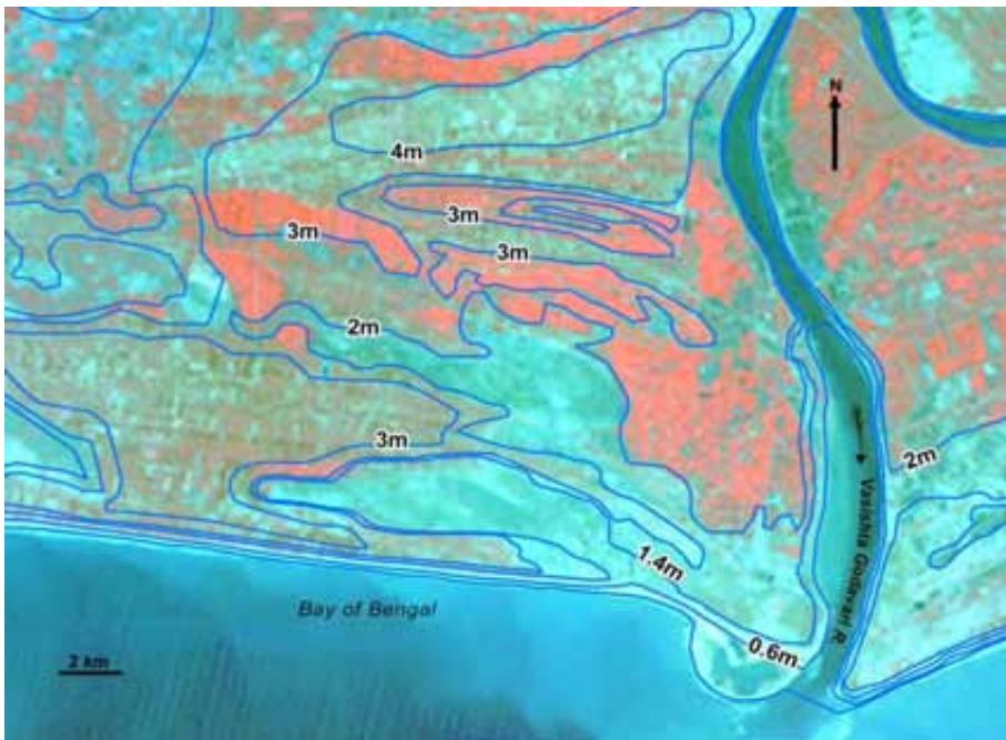
Fig. 7.17: Contours corrected using the landform patterns
