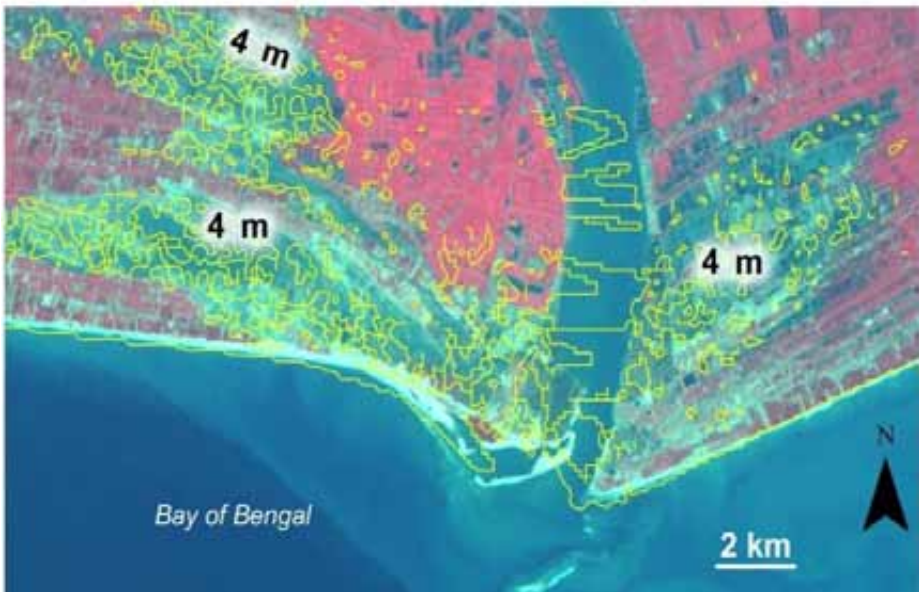
Fig. 7.16: Contours extracted from the SRTM DEM. Note the 4-m contour in the intertidal mudflats which in fact should be well within 2-m elevation
